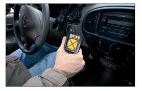
With the convenient hand-held control you can raise, lower and angle the plow from the comfort of your warm vehicle. A compact, dash mounted "joystick" is also available.
