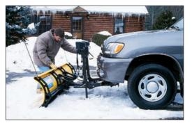
Attaching your Homesteader snowplow is so simple. Either drive into the attachment arms on the plow, or slide the Homesteader into the receiver brackets on your vehicle. Then connect two pins, remove two jacks, and plug in the electrical connectors.
