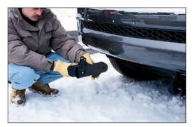
The receiver brackets on your vehicle are removable, by simply pulling the pins, for optimum ground clearance when you're not plowing.
