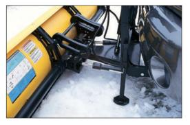
Heavy duty elastometer trip springs allow the blade to "trip" forward when it strikes an obstacle, protecting your vehicle and plow from jarring damage.
