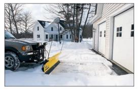
Exclusive Scrape Lock feature hydraulically locks the blade down for clean scraping action.
